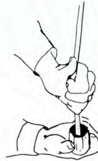
25. Removing burrs from tubes
