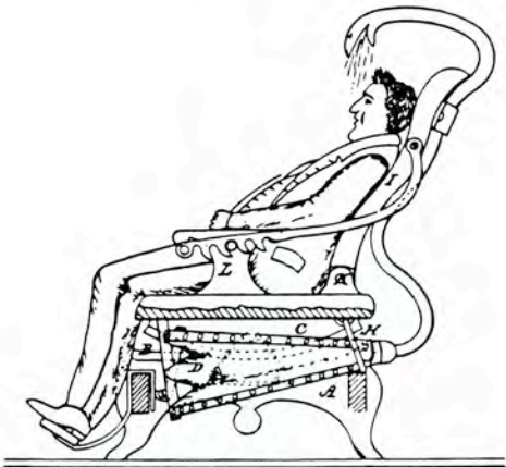
Rocking motion operates bellows
