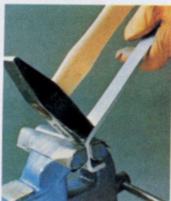
10 Bending metal sheets
