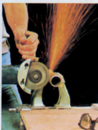
23 Grinding blunt (=dull edged) tools
