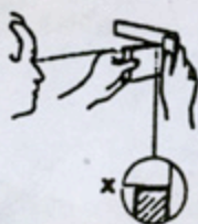
20 Checking right angles
