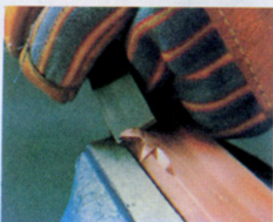
21 Scraping metal surfaces
