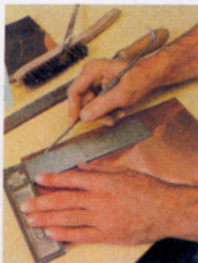
4 Scribing lines or circles on metal surfaces
