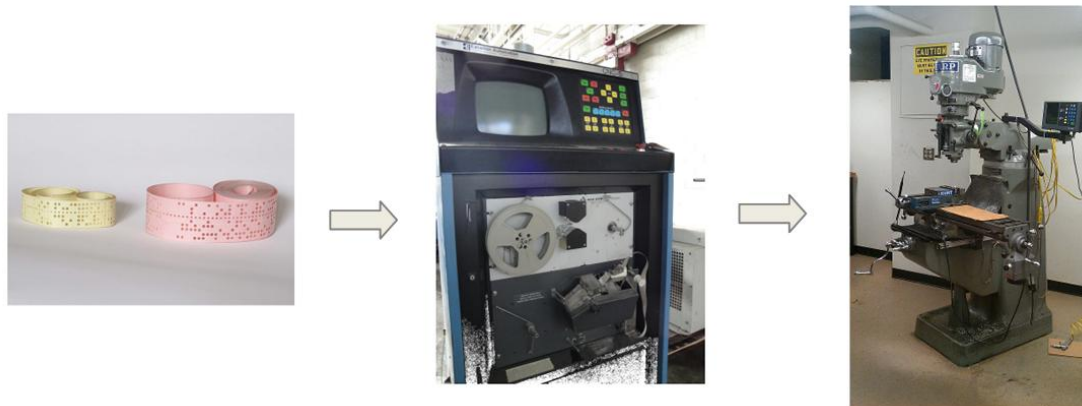
Σχήμα 2.36 Διαγραμματική παράσταση των βασικών στοιχείων συστήματος NC ( PaperTapes-5and8Hole by TedColes - Own work. Licensed under Public Domain via Commons, " Paper tape reader on a CNC control 001 " by Three-quarter-ten - Own work. Licensed under CC BY-SA 3.0 via Commons, Sharp 3 Axis Vertical Mill Full View by BUEngineer - Own work. Licensed under CC BY-SA 3.0 via Commons).
