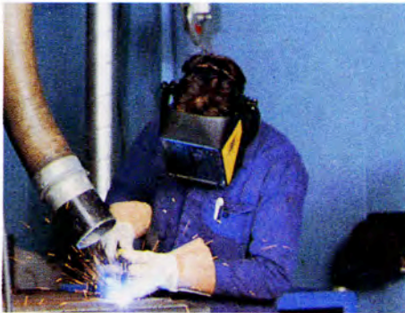
Proper dressing for the job to be done (overall, fire-proof gloves, face shield and shop cup)
