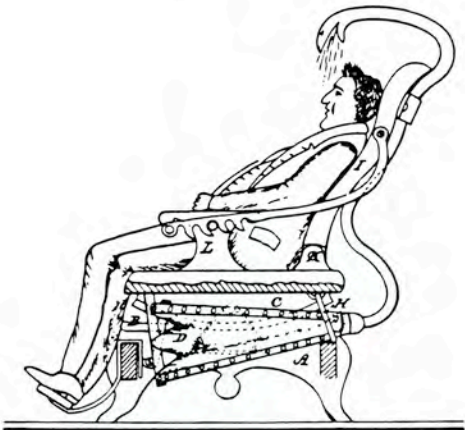
Rocking motion operates bellows
