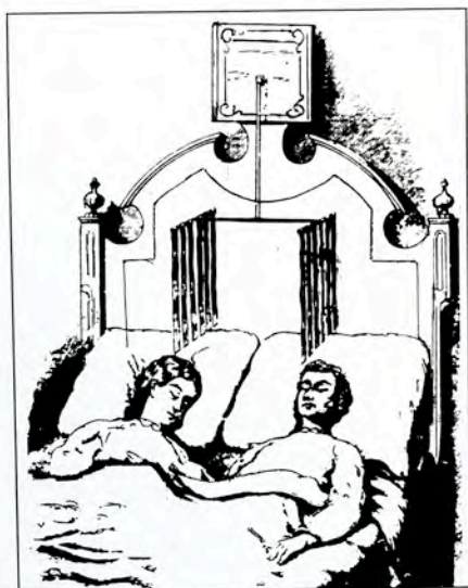
Clock mechanism moves fan device
