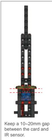
Keep a 10~20mm gap between the card and IR sensor.
