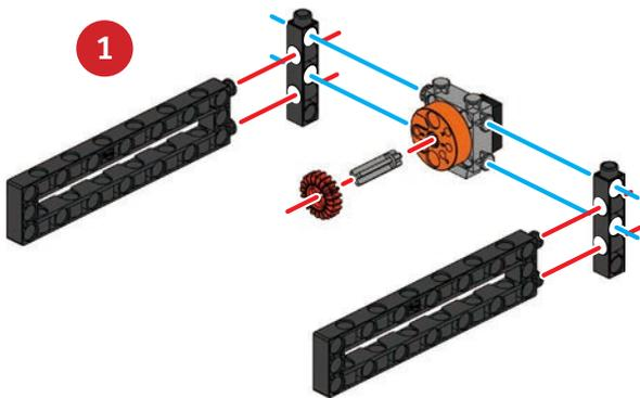
How to adjust motors to vertical position
