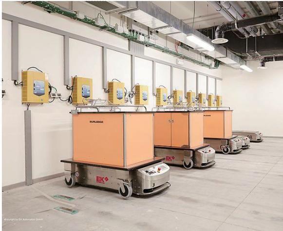
Powered Trams can run automatically and travel along a planned track on the ground. Using an infrared emitter, and infrared photoelectric crystal sensor the intensity of the reflected light determines whether the tram is on course. A controller is used to correct and adjust movement directions of the vehicle so that it can continue to run automatically on the track.
