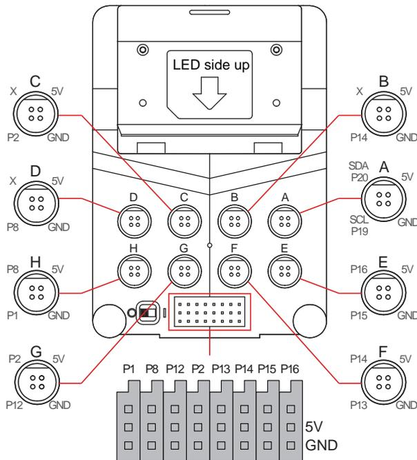
I/O pin configuration diagram
