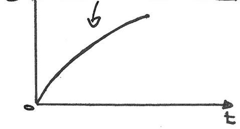
$$\omega = \omega_0 - \alpha_{\gamma\omega\omega} t \xrightarrow{\omega=0} t_{0n} \quad \Theta = \omega_0 t - \frac{1}{2} \alpha_{\gamma\omega\omega} t^2 \rightarrow t_{0n} = \frac{\omega_0}{\alpha_{\gamma\omega\omega}}$$
